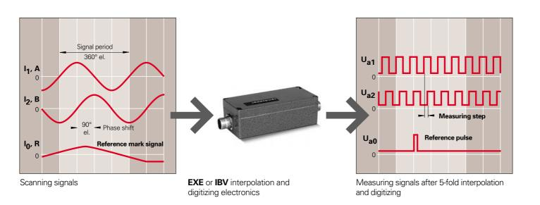
The inverse signals  $U_{a1}$ ,  $U_{a2}$  and  $U_{a0}$  have been omitted from the illustration to improve clarity.
