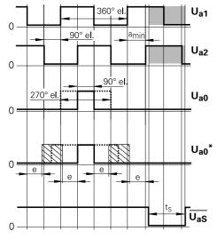
**Incremental signals:** Square-wave pulse trains  $U_{a1}$  and  $U_{a2}$  and their inverted pulse trains  $\overline{U_{a1}}$  and  $\overline{U_{a2}}$  (according to RS-422).
