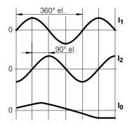
Sinusoidal scanning signals — preferably from HEIDENHAIN linear and angle encoders.
