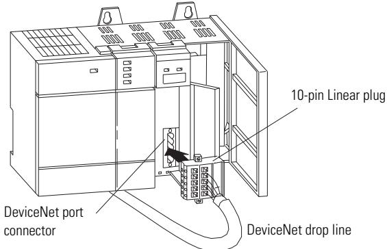
You have installed and wired your module. To operate the module you must apply power and then configure and program the SLC processor to communicate with it.
