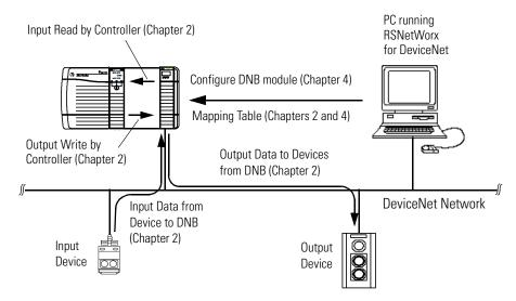
The 1756-DNB interface module can also be used to bridge a DeviceNet network with another network. See the referenced chapters for information on a particular topic.
