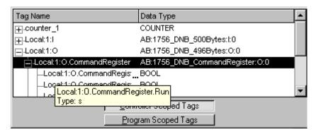
This output is the RUN bit for the 1756-DNB module in the local chassis, slot 1.
