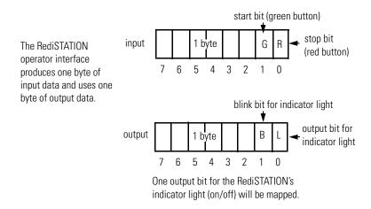
In the RediSTATION's bits for the red and green buttons and the indicator light status bit:
