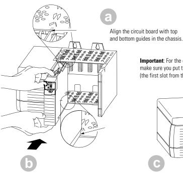
Slide the module into the chassis. Make sure the module properly connects to the chassis backplane.
