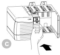
The module is fully installed when it is flush with the power supply and other installed modules.
