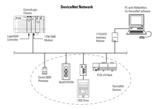
The 1756-DNB module communicates with DeviceNet devices over the network to:
