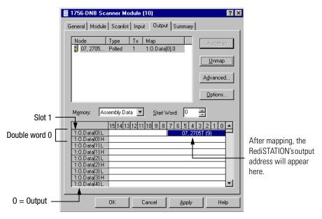
In this example, the output to the RediSTATION is mapped to double word 0 for slot 1 as the lower byte (bits 0-7) of the low word. Recall from chapter 2 that the indicator light is output bit 0. Therefore, the address for the RediSTATION indicator light is:
