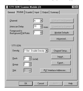
**4.** Make sure the 1771-SDN module's **Rack** and **Group** numbers are correct. We used Rack 0, Group 1 for the example application.
