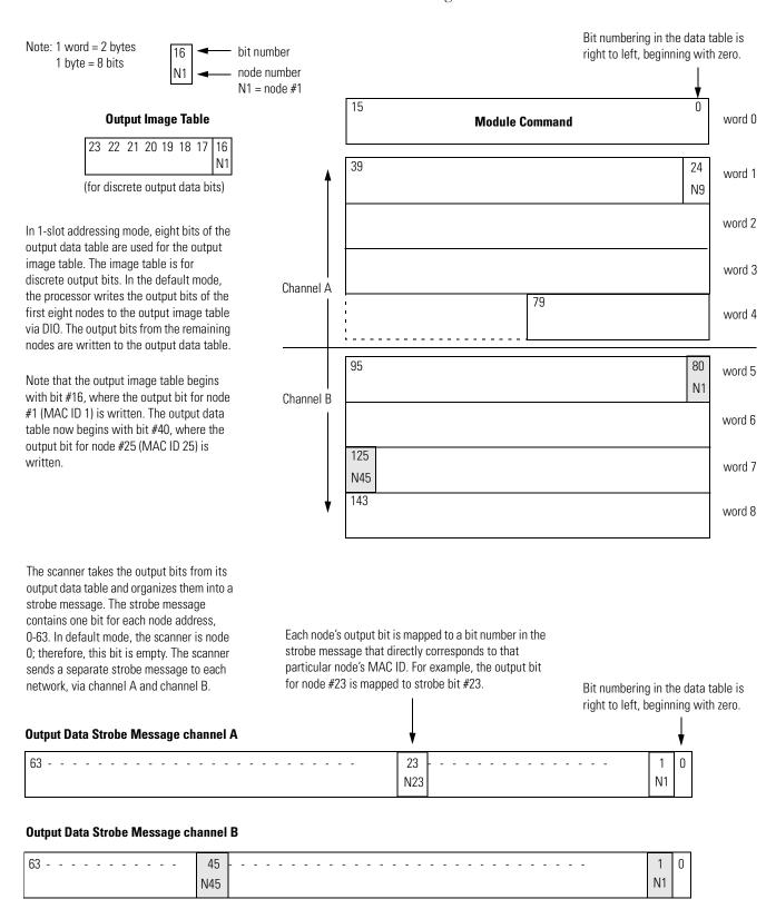
The following is an output data mapping scheme example for a scanner in 1/2-slot addressing mode.
