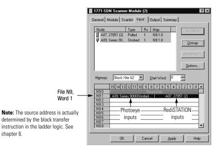
In this example, the input byte from the RediSTATION will appear in the PLC-5 processor in file N9, word 1, as bits 0-7. Recall from chapter 2 that the START button is bit 1 and the STOP button is bit 0. Therefore, the addresses for the RediSTATION inputs are:
