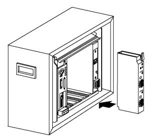
Apply firm, even pressure to seat the module in the I/O chassis backplane connectors.
