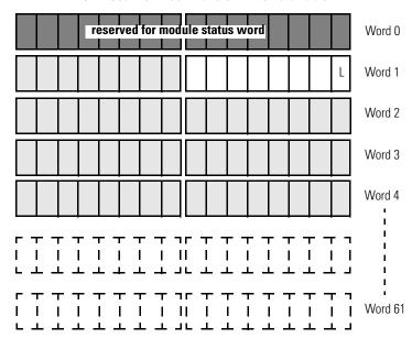
**Example:** The RediSTATION's indicator light (L) is taken from N10:1/0 in the PLC-5 processor's output data file.
