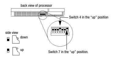
**2.** Set the baud rate to 57.6 Kbaud by placing switch 7 in the up position.
