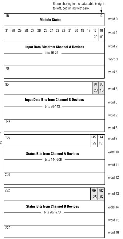
In 1-slot addressing mode eight bits are available for discrete input mapping, as shown below.
