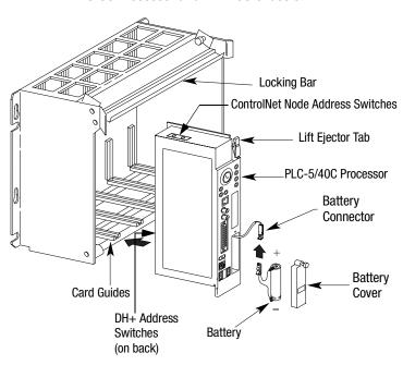
PLC-5C Processor and 1771 I/O Chassis
