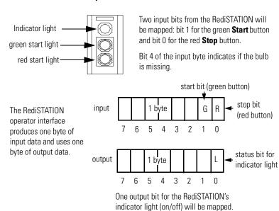
In the RediSTATION's bits for the red and green buttons and the indicator light status bit:
