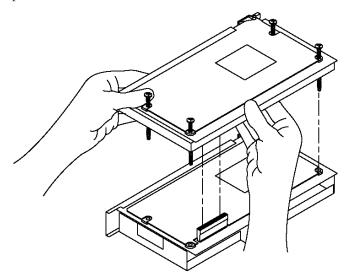
**3.** Insert the interface module/processor combination in the left-most slot of the 1771 I/O chassis.
