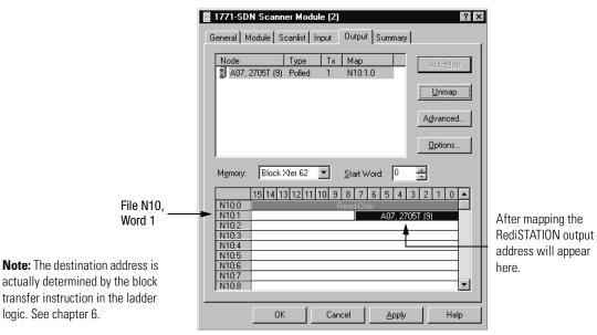
In this example, the output to the RediSTATION appears in the PLC-5 processor in file N10, word 1, as the lower byte (bits 0-7). Recall from chapter 3 that the indicator light is output bit 0. Therefore, the address for the RediSTATION's indicator light is:
