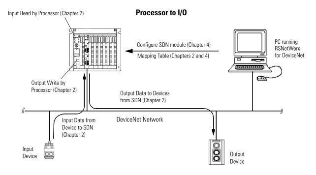
The 1771-SDN scanner module can also be used to bridge a DeviceNet network with another network.
