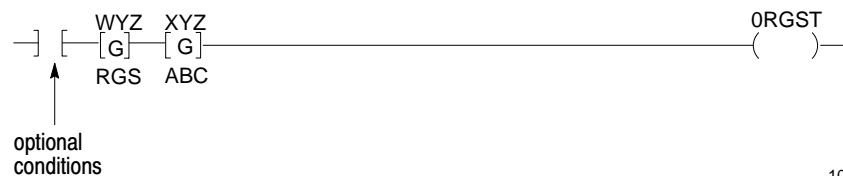
Figure 18.9 Block Transfer Rung
