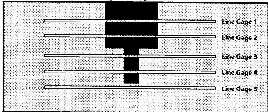
Figure 3.8 Stripped Wire Image Showing Line Gage Placement
