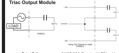
**Output Rating:** 24 VAC, 0.5 A (Cannot switch DC Loads)
