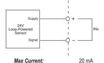
Voltage Supply to Sensor: 19 - 26V
