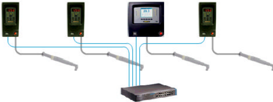
The figure shows a Cell that is created by using three Compact units, one Graph unit and a hub.
