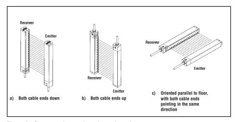
Figure 9. Correct emitter and receiver orientation
