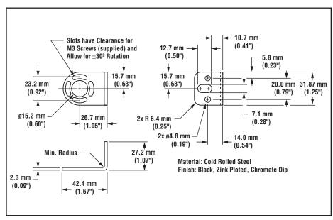
Figure 13. Emitter and receiver mounting bracket dimensions
