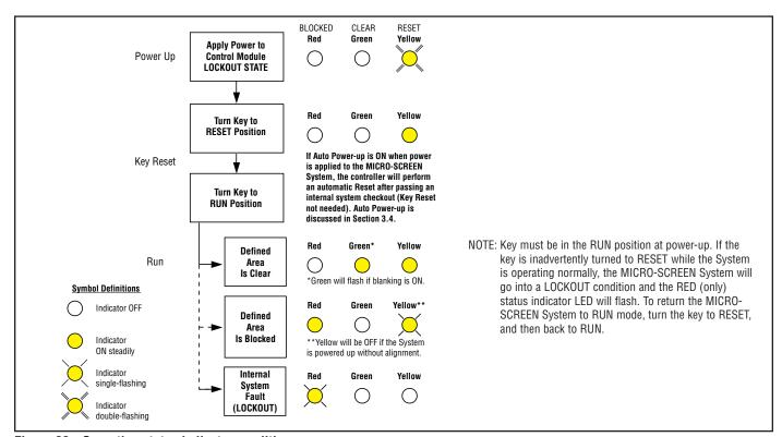
Figure 22. Operating status indicator conditions
