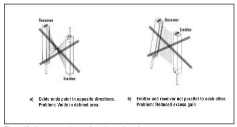
Figure 10. Incorrect emitter and receiver orientation
