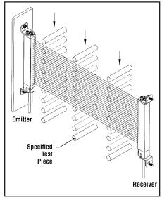
Figure 30. Use of test piece in trip test
