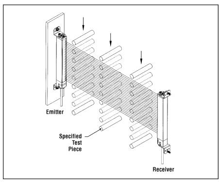
Figure 27. MICRO-SCREEN trip test
