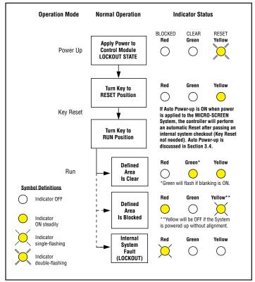
Figure 25. Operating status indicator conditions
