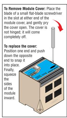
Figure 19. Control module cover removal
