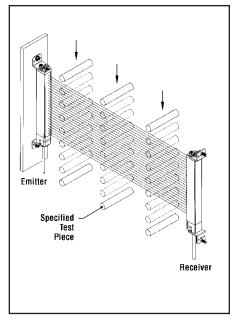
Figure 23. MICRO-SCREEN System trip test
