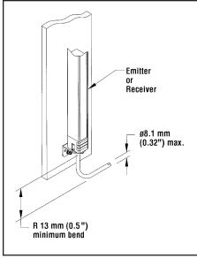
Figure 16. Cable clearance dimensions
