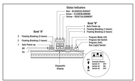
Figure 20. Controller board configuration DIP switches
