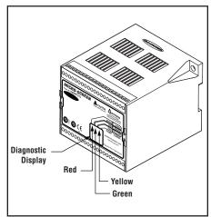
Figure 4. Control module indicator LEDs
