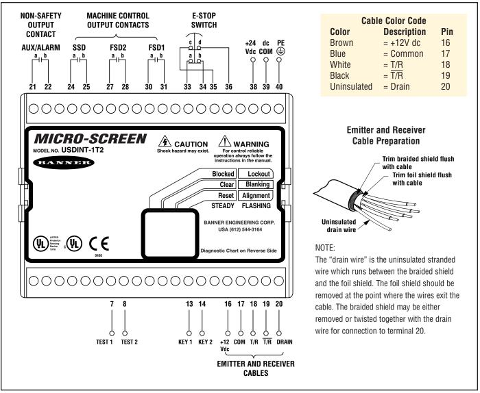
Figure 21. MICRO-SCREEN System electrical connections
