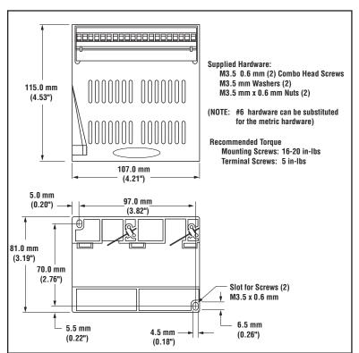
Figure 17. Control module dimensions and mounting hole locations
