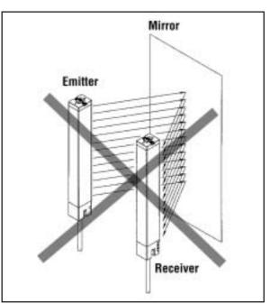
Figure 11. Never use MICRO-SCREEN sensors in retroreflective mode.
