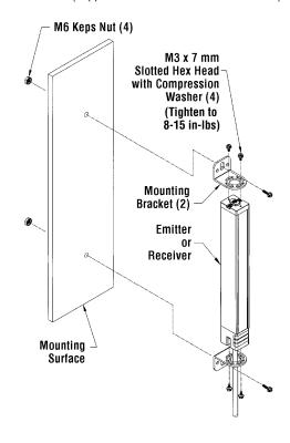
NOTE: MICRO-SCREEN sensor brackets are designed to mount directly to MSA Series stands (page 61), using the hardware supplied with the stands.
