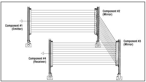
Figure 28. Corner mirror alignment
