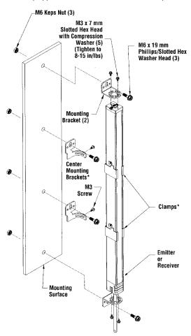
\* 40" to 48" sensors include one center bracket and clamps to be located at the midpoint along the sensor's length
