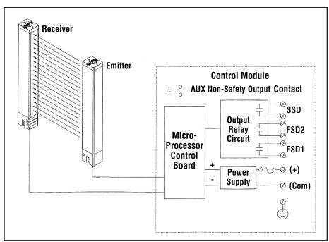
Figure 6. Banner MICRO-SCREEN System functional schematic
