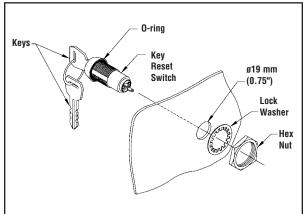
Figure 18. MICRO-SCREEN Key Reset switch mounting
