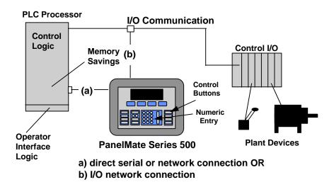
PanelMate Series 500 performs all the same control and monitoring functions as the devices on a hard-wired operator station, plus adds many more capabilities. It also:
