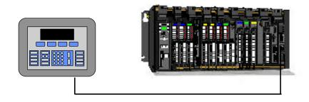
This means that PanelMate Series 500 does not directly connect to PLC I/O points except when it is operating on a PLC's remote I/O network. PanelMate Series 500 is usually the "master" device when it communicates to the PLC. This means that:
