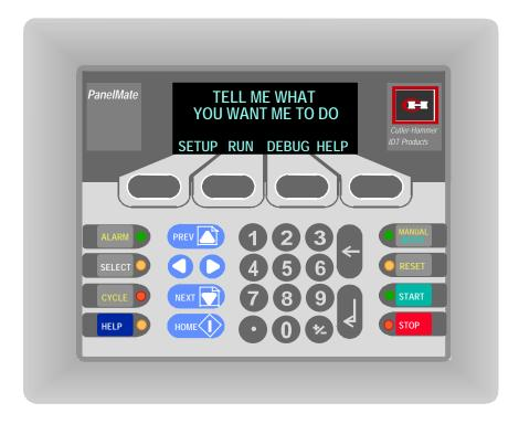
The unit illustrated above features a 4-line text display area, which is available as either vacuum fluorescent or LCD display type. PanelMate 500 is also available in 2-line vacuum fluorescent or LCD display versions.
