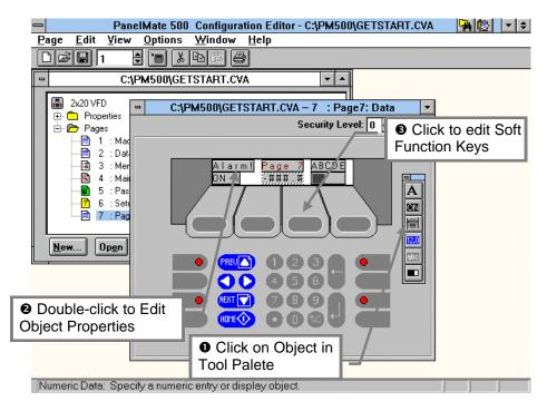
As shown in the following illustration, after selecting a bar graph object from the tool pallette, the bar appears at the top left of the display. When the cursor is double-clicked on the bar, the bar graph properties spreadsheet will appear. In this same fashion, any of the other 5 object types may be added to a data page.
