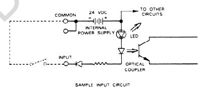
Figure 6-8. Wiring for 24 V ac Sink Inputs
