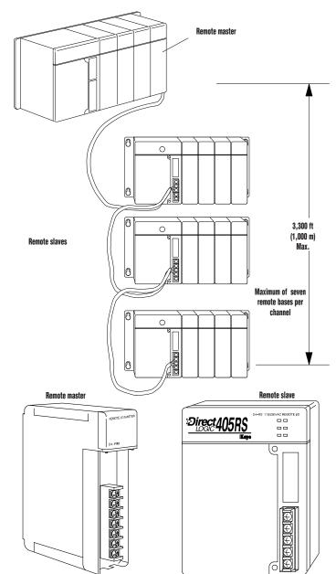
You can assign normal input and output addresses to the remote points, or you can assign special remote I/O addresses. The Remote Master sends the remote I/O information to the CPU. The communication between the Remote Master and the CPU is asynchronous to the CPU scan. For this reason, remote I/O applications should be
