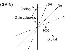
Gain is the angle or slope of the calibration line identified at a digital value of 1000.
