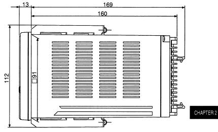
Recommended thickness of mounting panel: 1 to 8 mm
