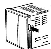
Pull out the body while pushing in the catch at the bottom of the controller.
