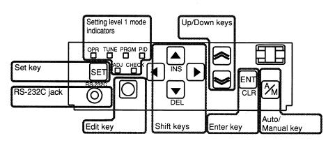
Setting level 1 mode indicators The LED corresponding to the mode set in setting level 1 lights. Correspondence between the LED and setting mode is as follows:
