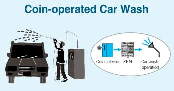
The ZEN can be used to change the operating time depending on the number of coins inserted. If a holding timer (#) is used with holding bits (H) in self-holding programming, the remaining time will not be reset even if there are unexpected power interruptions.
