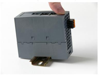
Figure 4-1 Installation on a 35 mm DIN rail
