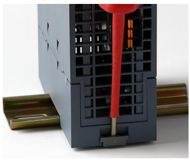
Figure 4-3 Removal from a 35 mm DIN rail
