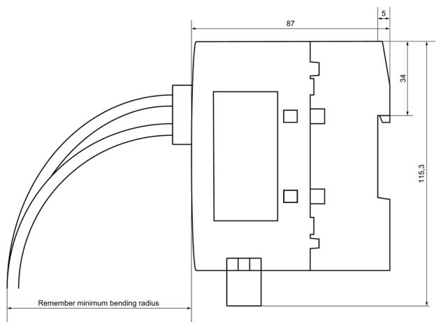
Figure 9-2 Dimension drawing, side view (example: SCALANCE XB004-1)
