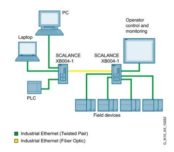
Figure 2-2 Example of an electrical/optical star topology with SCALANCE XB004-1
