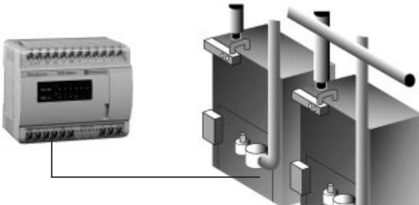
TSX Nanos with 16 and 24 I/O have 16 schedule blocks, for which internal and external outputs can be defined.
