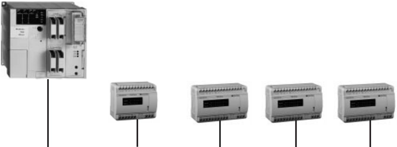
*Up to four TSX Nano PLCs can be connected as remote I/O without programming. Three TSX Nanos can be connected for remote processing.*
