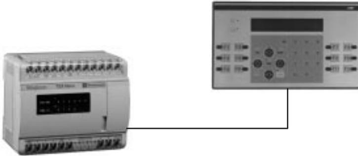
A display is continuously available to the operator, providing information on the production process. In real time, the user can intervene as soon as an anomaly appears. The operator terminal, connected to the TSX Nano terminal port can:
