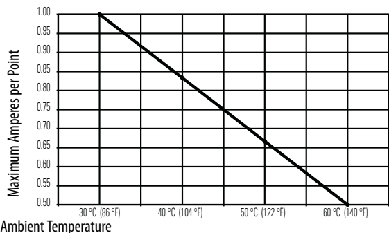
Figure 2 - Embedded DC Outputs Maximum Amperes per Module Versus Temperature
