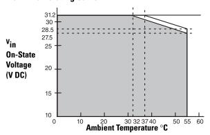
The area within the curve represents the safe operating range for the module under various conditions of user supplied 24V DC supply voltages and ambient temperatures.
