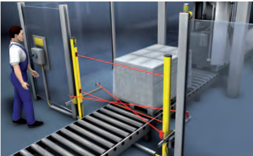
The ASM Muting functionality enables pallets in a wrapping machine application, for example, to pass by the active opto-electronic protective device without any process interruption.
