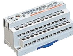
FN-Y16SC41 16-point Discrete Source Output
