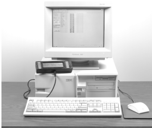
Control module connected to PC via AS42CM-SC cable
