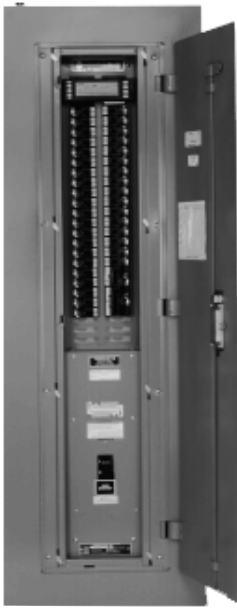
POWERLINK AS panelboard with 1-, 2-, and 3-pole series-rated circuit breakers with high interrupting 250 amp main circuit breaker.
